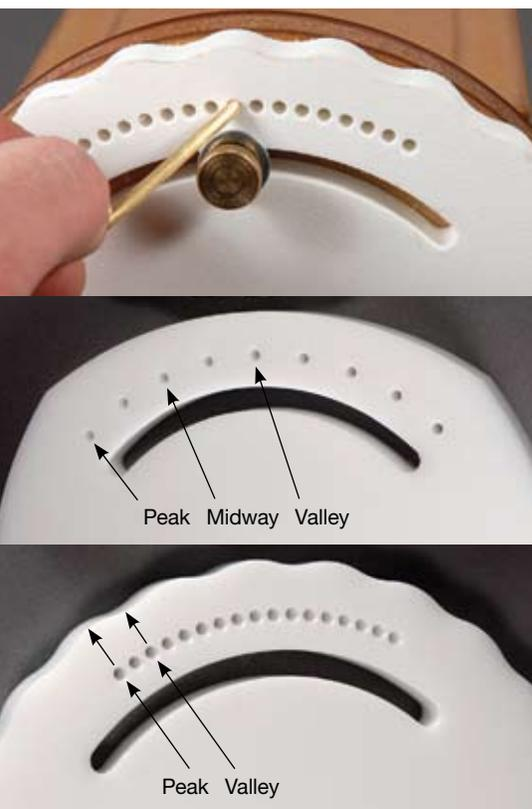
**Top:** Insert a pin through the phasing hole on a rosette. Note that the pin will be aligned with a peak of the 24-lobe rosette.
