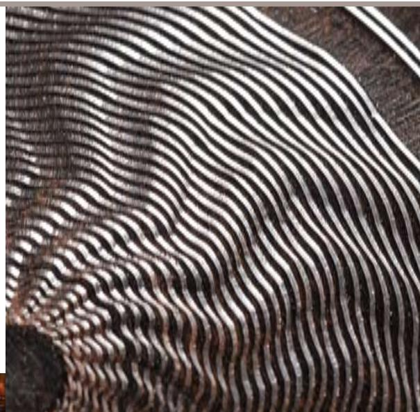
*Above:* To produce the moiré pattern, the notch plates or phasing holes are moved forward a few, then back a few. This moiré example is turned with a fixed cutter on African blackwood end grain.
