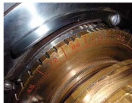
A typical notch plate on an antique rose-engine lathe shows the predominant multiples of 12, and the small number of notches actually required for each group.
